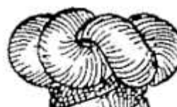
FIG. 113.—Single crown tucked (complete).
