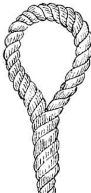
FIG. 90 B.—Flemish eye (complete).
