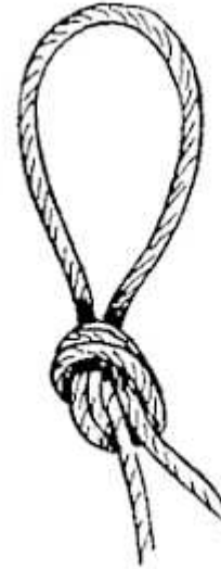
FIG. 62.—Loop knot. FIG. 63.—Loop knot.
