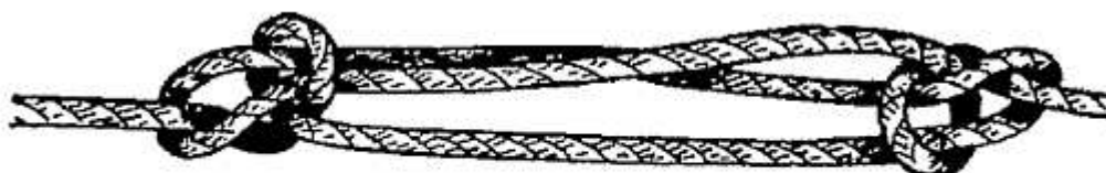
FIG. 82.—Sheepshank for free-ended rope.
