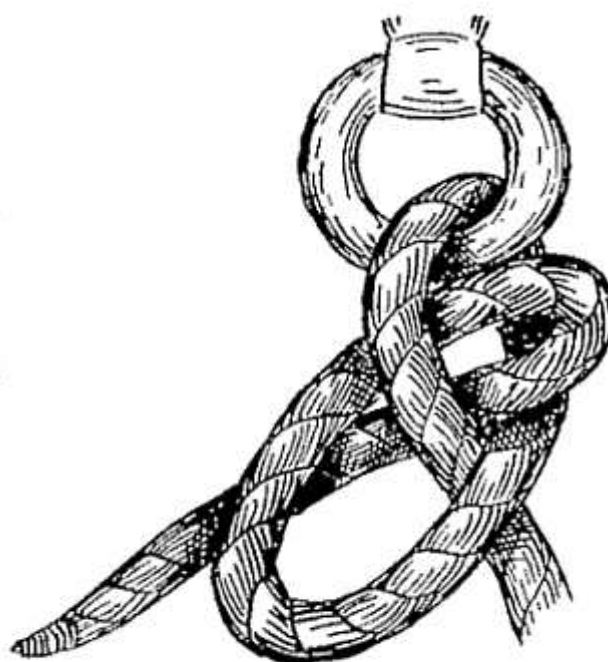
FIG. 33 —Slippery hitch (tying).
