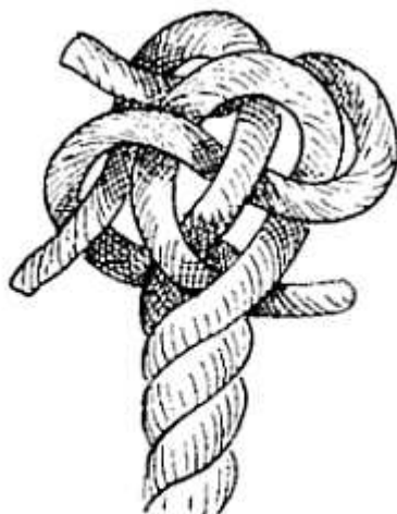
FIG. 121 A.—Making double crown.
