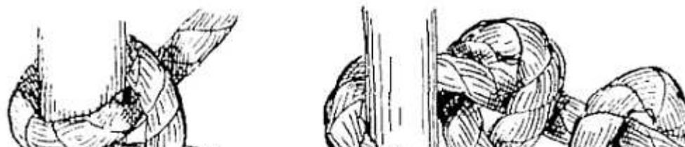
FIG. 33 —Slippery hitch (tying).
