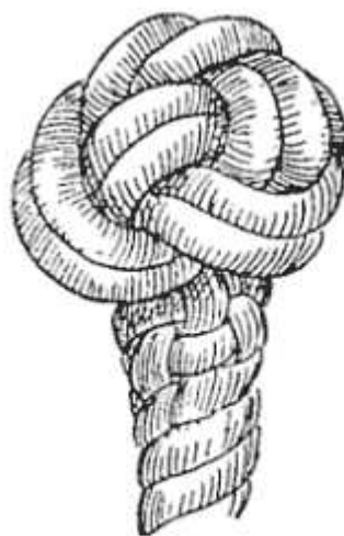
FIG. 127.—Double wall and crown (complete).
