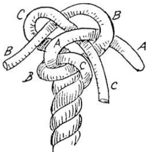
FIG. 124.—Wall crowned (making).
